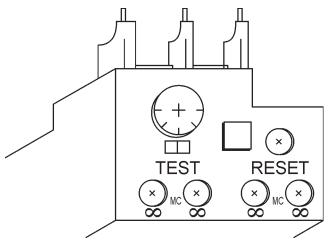
Figure 11. Over Current Relay
